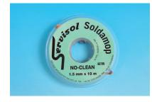
SOLDAMOP NO-CLEAN is manufactured using high purity oxygen free and oil free fine gauge copper wire. It is impregnated with a special 'No-Clean' flux. This flux significantly improves the wicking action of the braid. The residue left behind is halide free and non-conductive which means it does not need to be cleaned off.
