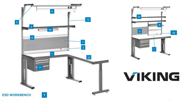
These workbenches can be placed in a line to make a common working area with no gaps. Universal design allows fitting out the workplace with necessary equipment and drawer units. Load capacity: 200 kg. Height adjusment: 800 - 950 mm Temperature restistance: 300 ° C
