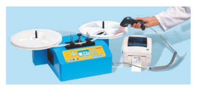
For taped SMD component counting. This machine works in a simple way by counting the holes on the tape.
