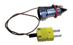
⇒ K-Type thermocouple and subminiature connector assembly with ZD13 desoldering tip and RS383 retaining sleeve attached (use as a calibration aid with MS412 temperature measuring system)
