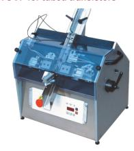
SUPERCUT/TOCF automatic machine is designed to cut and form tubed radial components type TO220, TO218, TO126. The complete operation is fully automatic and each form needs dedicated die. The full tube is introduced into the
