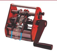
SUPERFORM/A-LC is a machine made for cutting and bending axial taped components, it is extremely compact and sturdy and its main characteristic is to form components with rheophore up to 1.4 mm
