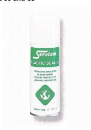
PLASTIC SEAL 60/65 Protective coating for PCB's and electronic components. Cures on exposure to air leaving a thin insulating film which protects against humidity, air pollution and environmental attack. Film can be soldered through to facilitate 'spot' repairs.
