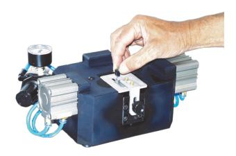
A pneumatic machine designed to cut loose radial component leads. The feed is manual, on the top of the machine. Pressing the footpedal effects cutting and prefoming of the leads in a very quick and precise way. A large variety of Dies is available, substitution of the Die assembly is extremely quick and simple. A machine three cylinders equipped, with custom tool, can be supplied for more complex not standard forms.
