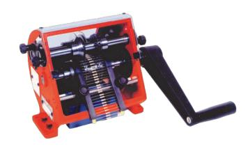
SUPERFORM/AP is a machine made for cutting and bending axial taped components for vertical assembling, and shaping a little curl on each lead. The machine handles wire diameters ranging from 1 mm to 1.4mm. By replacing the 2 .cutting/forming wheels. with 2 .only cutting wheels. (optional) it is possible to obtain an U-shape without curls.
