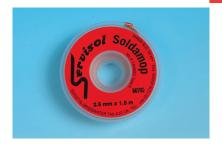
SOLDAMOP is manufactured using high purity oxygen-free and oil free fine gauge copper wire. The wire is specially impregnated with flux, which cleans thoroughly during the desoldering process. The flux coating also provides long lasting protection of the copper wire from the effects of oxidation.
