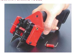
This tool is hand operated, adjustable, useful to obtain a U-form for axial components.
