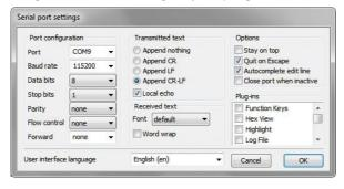
The "Port" field must contain the virtual serial port number assigned to the device for proper operation.
